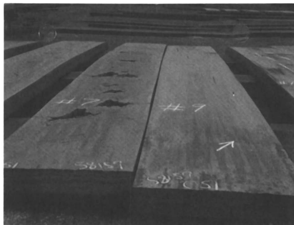
Figure 3. Hot shortness—large and deep tears and holes in a slab of carbon steel treated with 6 lbs of mischmetal per ton instead of 2 lbs, by accidental malpractice
